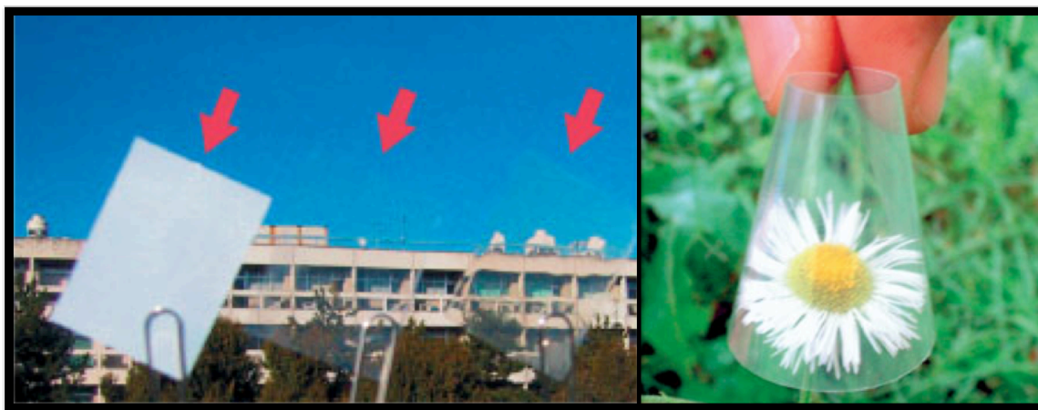
Figure 7: Transparent and flexible BC sheet. (adapted with permission from Yano et al. 2005)
