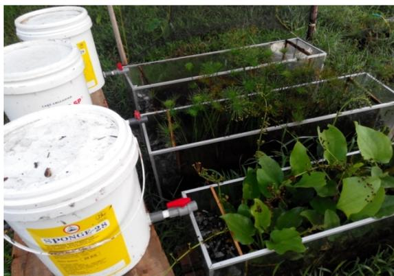
**Gambar 1.** Reaktor *Sub-surface Constructed Wetland*
