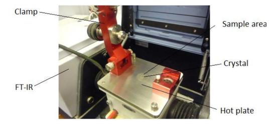
Figure 2.9: An example of a Golden Gate ATR accessory with a thermal top plate.
