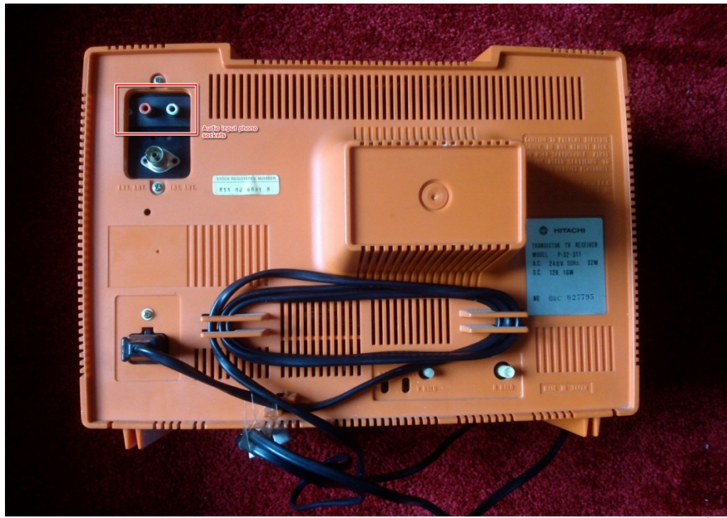
Figure 11: Rear of the Hitachi P-32-311 TV showing audio input
