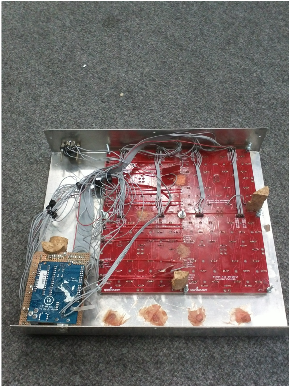
Figure 3: Internal view of Arduinome
