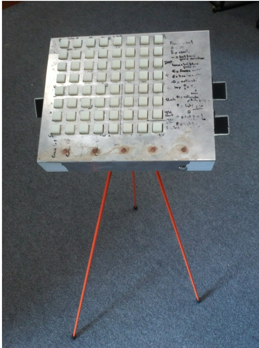
Figure 1: Arduinome mounted on repurposed surveyors' tripod
