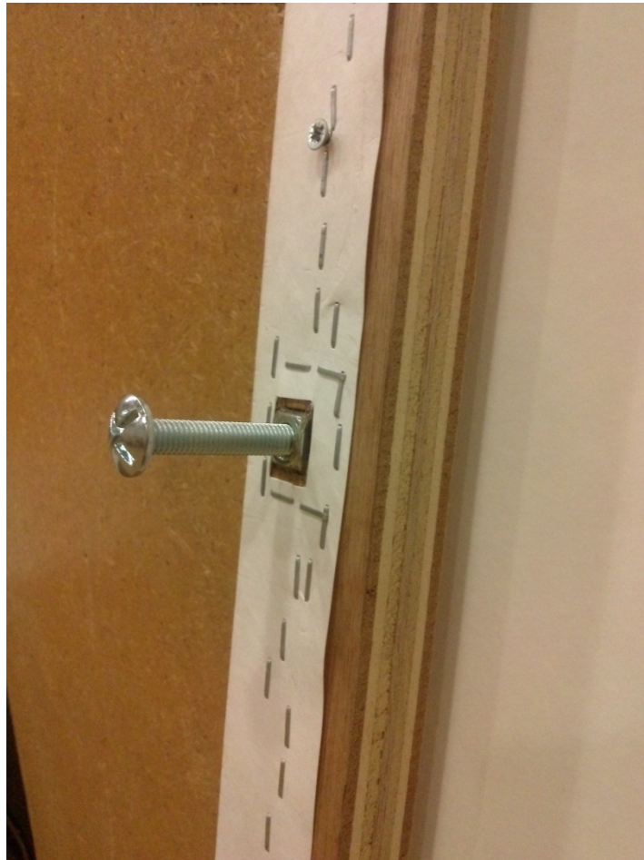
Figure 8: Close up view of LaFPanS tensioning bolts
