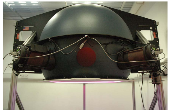
Fig. 2. RS-5B optical heads mounted onto the 1 m integrating sphere.
