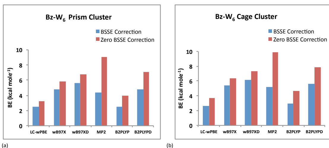
Figure 3. Variation of BE's (kcal mol -1 ) (with and without BSSE correction) of Bz-W 6 clusters versus different DFT hybrid functionals and MP2 method (a) prism conformer (b) cage conformer.
