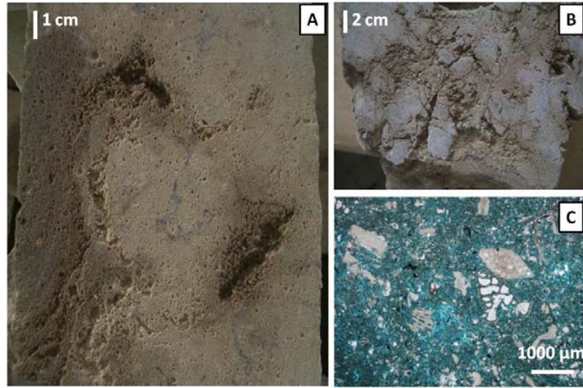
Fig. 8 Illustration of varying scales of solution-enhanced porosity caused by late-burial corrosion within the CEP zones in A and B Zones. (a) Vuggy/moldic porosity in core. (b) Leached stylolite and associated tension-gashes. (c) Matrix micro- and macro-porosity observed in thin-section.
