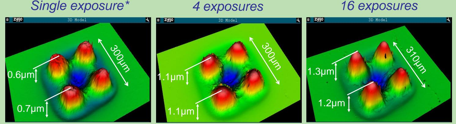
\* Single exposure = 13.33ms train of laser pulses at a 400kHz pulse rep-rate
