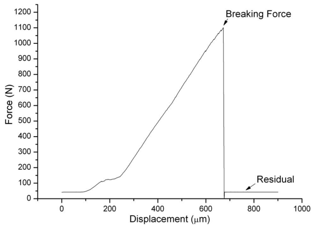
Fig. 6. Example plot of recorded shear force test. The shear force for the piece is calculated as the breaking force minus the residual force (due to the mass of the test rig being supported by the mechanism).
