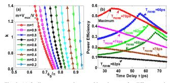
Fig. 2. (a) Scaling parameter k versus bias phase  $\varphi_b$  for different peak amplitude of the input Gaussian pulse (b) calculated power efficiency of the modified triplets for different input pulsewidth and time delay.
