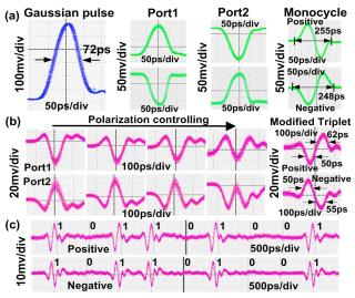
Fig. 4. (a) Gaussian-like pulse from PPG and generated monocycle pulses (b) evolution of the modified doublets and the obtained modified triplets (c) OOK modulated UWB signals with a pattern of "101101001".
