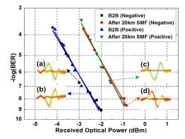
Fig. 6. BER curves and eye diagrams of the FCC-compliant UWB signals for B2B and after 20 km fiber transmission.
