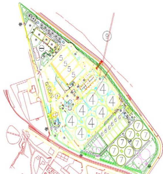
Fig. 5 Layout of Seafeld wastewater treatment plant: 1 is the screen house, 2 are the detritors, 3 Grit washing mechanism, 4 sedimentation tanks, 5 storm tanks, 6 aeration tanks, 7 final settling tanks, 8 UV treatment unit, 9 outfall tunnel
