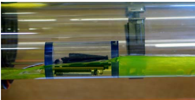
Figure 6. Cylindrical NBS solid in a flow
