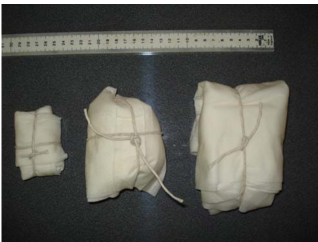
Figure 10. Formation of simulated large solids
