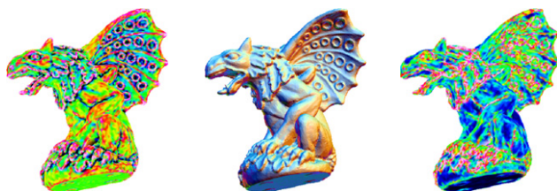
Fig. 3. Color encodings (please see the online version of this paper for this figure in color) for the mean curvature (left) and curvedness (right) detected on Gargoyle model (center).
