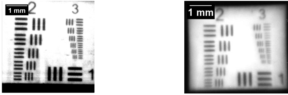
Figure 8. Resolution measurements using the infrared band-pass filter (3 to 6 microns) for: a) 50 \mu\text{m} , b) 25 \mu\text{m} , c) 10 \mu\text{m} CMIR-TI system scanning; d) MIR-TI measurement.
