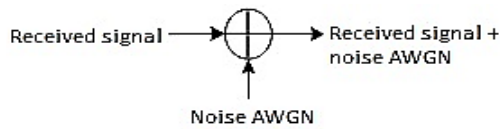
Fig. 5 Modelling of AWGN channel addition.
