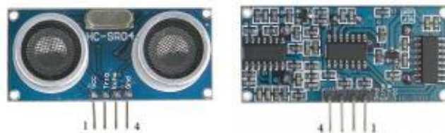
Fig. 1 HC-SR04 ultrasonic sensor, front (left), rear (right) (datasheet).
