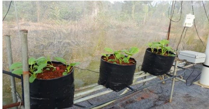
Figure 3. Experimental setup for the fibrous capillary irrigation with the IoT monitoring system
