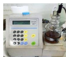
Figure 2. Instrument CA-21 measure water content automatically
