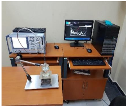
Figure 1. The loss factor measurement setup based on open-ended coaxial probe
