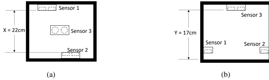
Figure 3. Ultrasonic sensors placement for item classification, (a) Top view, (b) Side view
