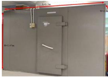
Figure 2. RF-shielded room for indoor measurement setup
