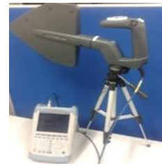
Figure 3. Antenna setup for far field BTS radiation exposure
