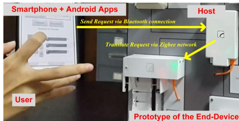
Figure 12. Setup for functional test result of curtain device
