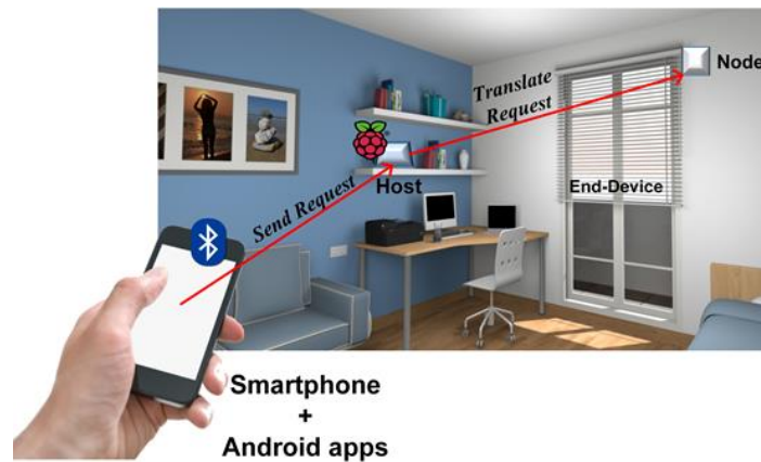
Figure 3. Architecture of the curtain control system
