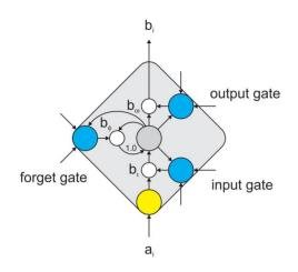
Figure 3. Structure of LSTM cell (Source: Sundermeyer, Schlüter & Ney, 2012)
