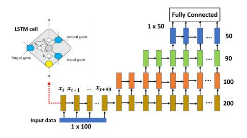
Figure 2. Structure of LSTM model
