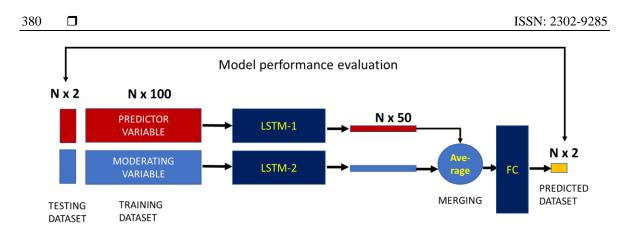
Figure 1. The structure of merged-LSTM model
