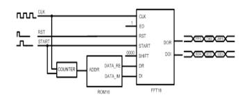
Figure 2. Pipelined FFT testbench
