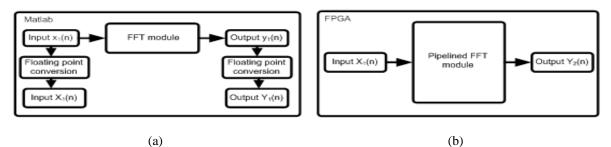
Figure 1. (a) FFT Module in matlab (b) Pipelined FFT module in modelsim
