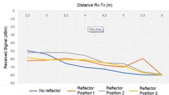
Figure 8. Signal reductions due to propagation and obstacle
