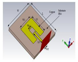
Figure 1. Top view of printed antenna
