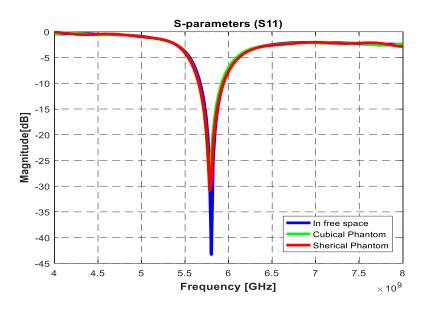
Figure 4. Comparison of the simulated reflection coefficient of the designed square ring antenna in free spaces and human head
