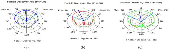
Figure 7. Comparison of Simulated Radiation characteristics of the proposed antenna (a) in free space (b) Cubical phantom and (C) Spherical Phantom at 5.8 GHz
