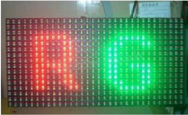
Figure 2. Three colors LED dot matrix panel
