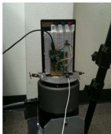
Figure 16. Test set up for Vibration test
