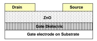
Figure 2. Bottom gate ZnO thin film transistor
