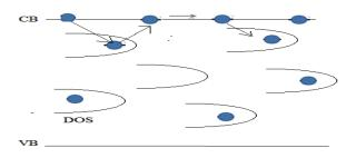
Figure 3. Multiple-tapping and release mechanism
