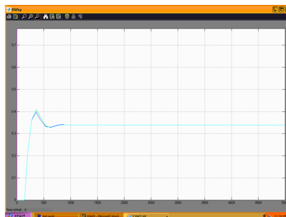
Figure 9. Output for varying input servo model for basis weight at different values of K_D
