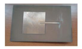
Figure 13. Fabricated Rectangular Microstrip
