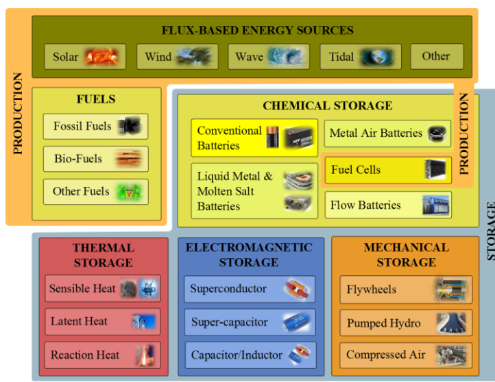
Figure 2. The landscape of energy/electricity generation and storage solutions (representative sample). It should be noted that fuel cells are a production technology but have been categorized as storage to adhere to common convention.
