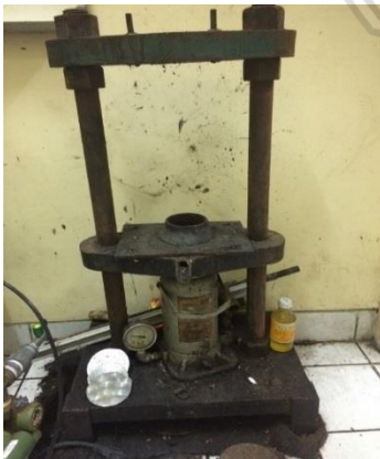
Gambar 3.6 Mesin press rubber seed oil
