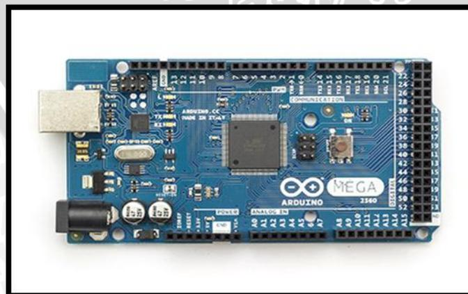
**Gambar 4.9** Arduino Mega 2560
