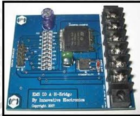
Gambar 4.7 Modul Driver Motor
