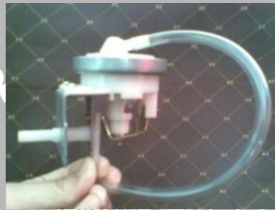
Gambar 4.6 Sensor Water Pressure Switch .
