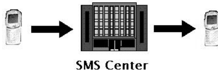
Figure 2.4. Basic concept of sending SMS
