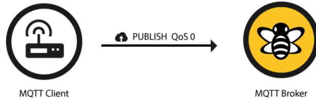
Gambar 2.12 MQTT QoS level 0
