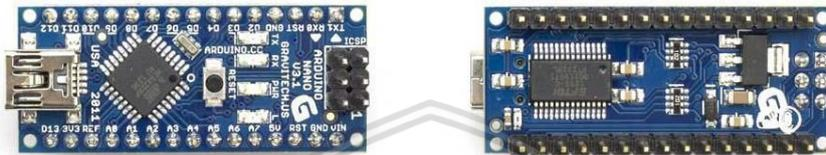
**Gambar 2.9 Arduino Nano v3.0**
