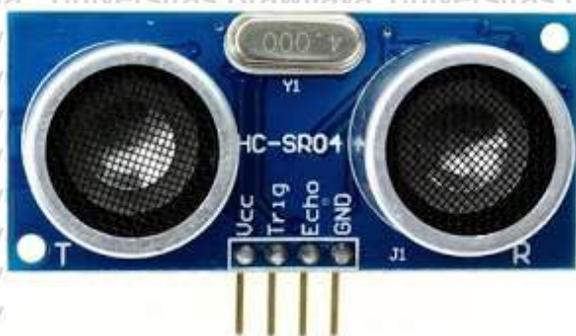
Gambar 2. 4 Sensor Ultrasonik
