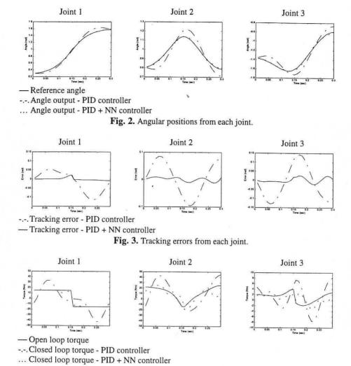
Fig. 4. Open-loop torque and closed-loop torque on each joint.
