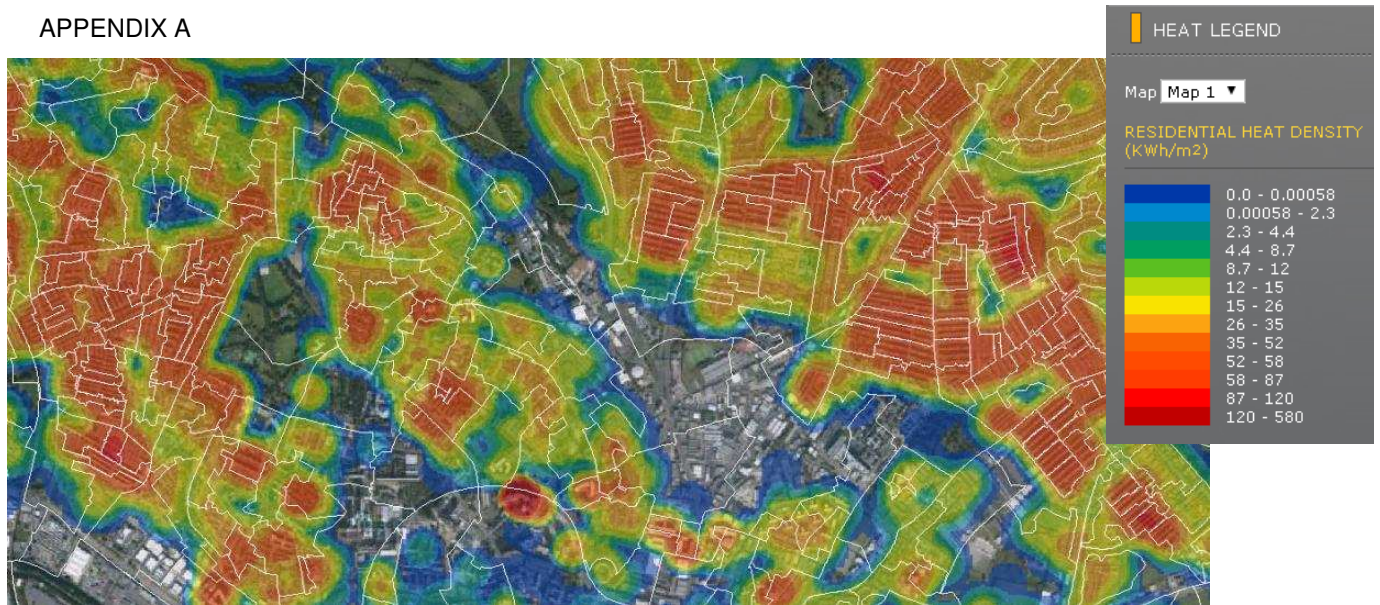
Fig. 1 Extract from the DECC National Heat Map showing modelled residential heat demand in Leeds, UK.
