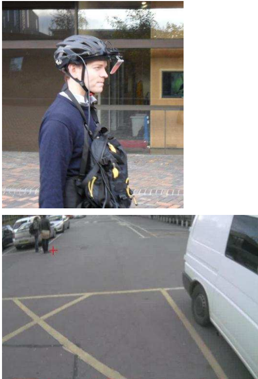
Figure 1. Eye-tracking apparatus and an example of the record – the red cross indicates fixation.
