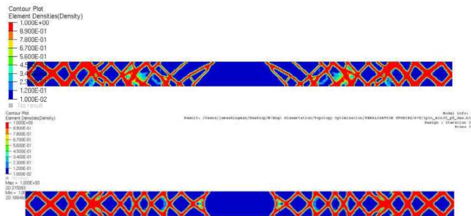
Figure 7 - a) Results of a topology optimisation study on a beam web; b) Results of a topology optimisation study on a beam web incorporating a symmetry constraint
