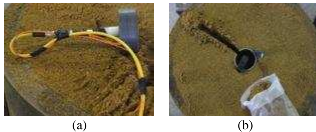
Figure 5. Images taken from charge preparation process: (a) non-el detonator and break-wire umbilical prepared for burial (b) charge hole and umbilical trench prepared
