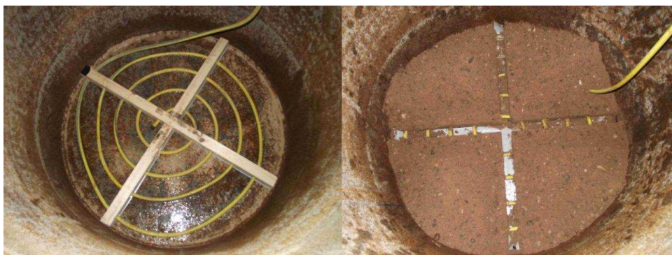
Figure 4: Bottom-up saturation technique a) spacer present b) part-filled with spacer removed
