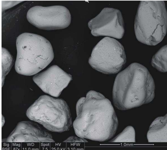
Figure 3: Scanning electron micrograph of Leighton Buzzard sand [6]
