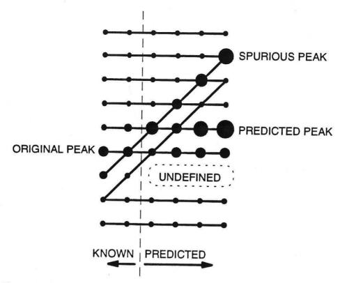
Figure 2: An example of the problems caused by inappropriate application of the basic FBP model.
