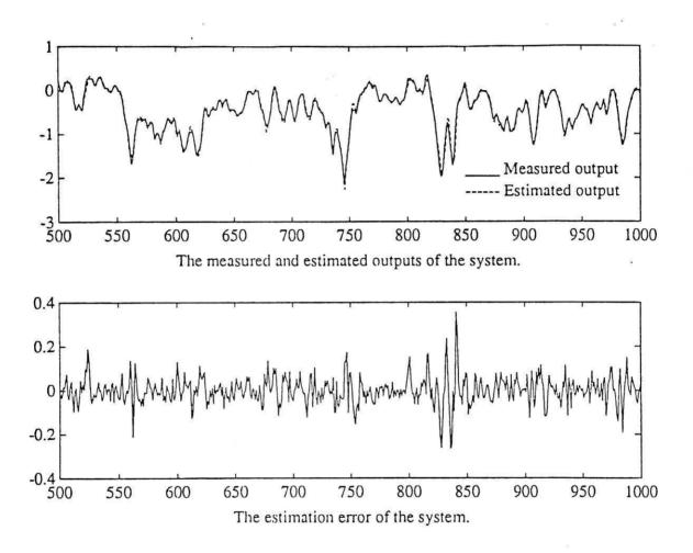
Figure 6: The validation results of the system using GRBF network.
