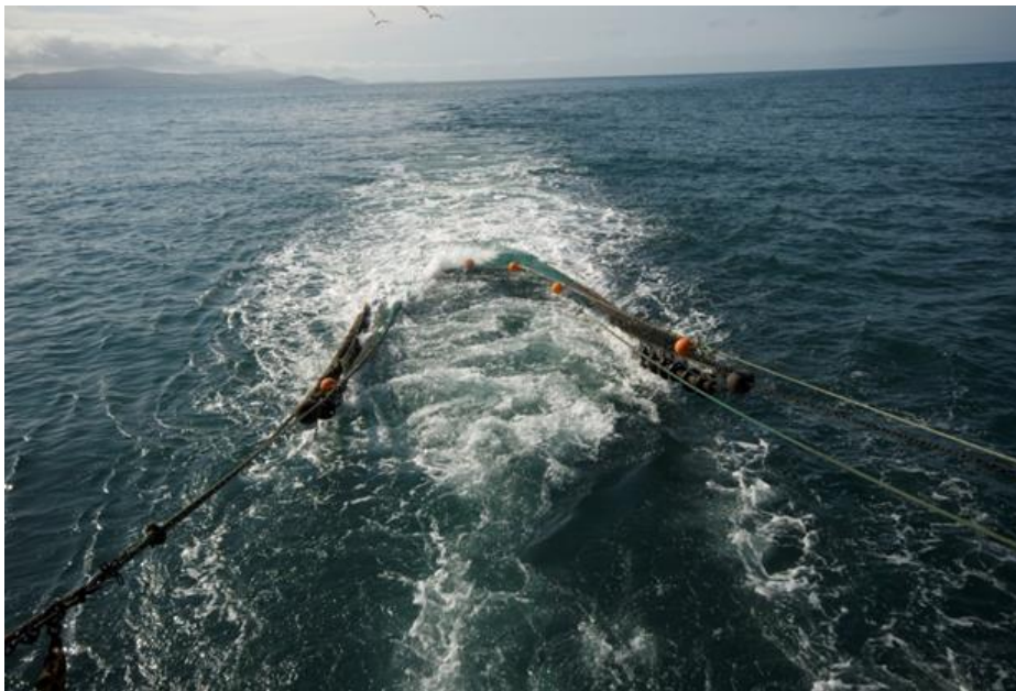
Figure 6 | A demersal otter trawl being retrieved with a catch of queen scallops ( photo: Simon Park )
