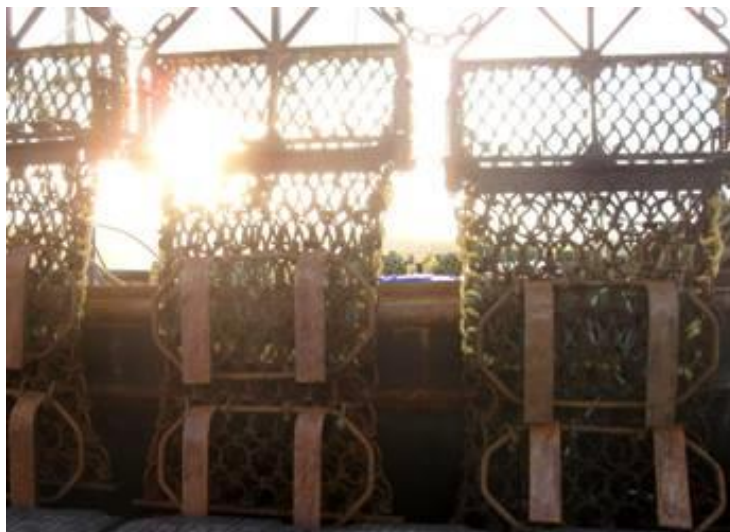
Figure 5 | A gang of skid or ski dredges showing the four skids on the underside of each dredge, but the absence of a toothed bar (photo: Harriet Salomonsen)
