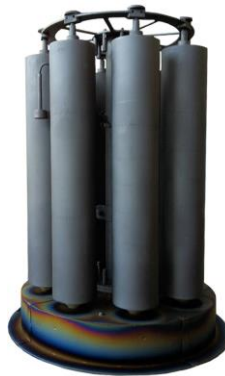
Figure 3-5: Image of the substrate table for the Hauzer Flexicoat 850 deposition system
