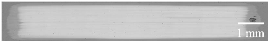
W-DLC in fully formulated oil + ZDDP after twenty hours
