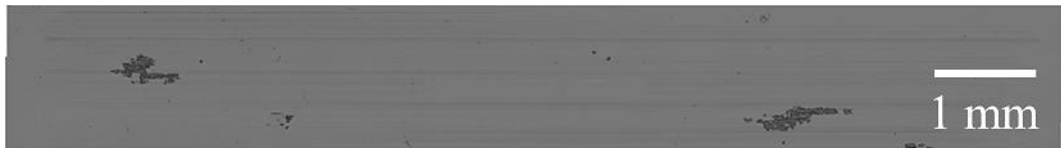
Si-DLC in fully formulated oil + ZDDP after six hours
