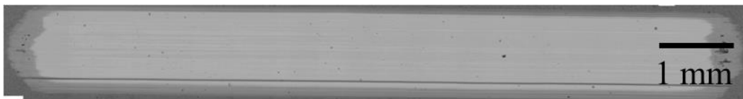
W-DLC in fully formulated oil + ZDDP after six hours
