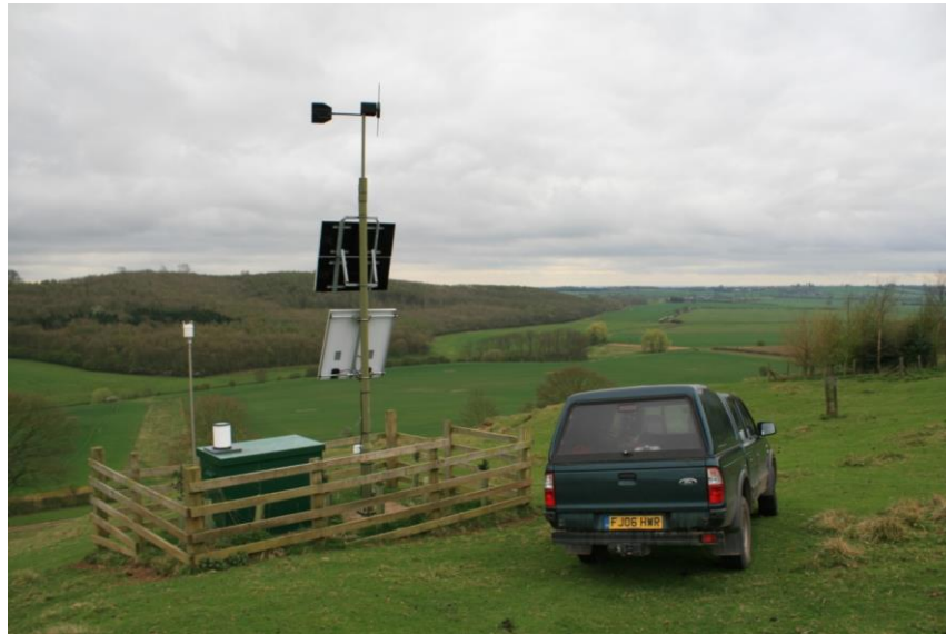
Figure 4.5. Position of rain gauge at Hollin Hill field site (white cylinder on roof of green enclosure).
