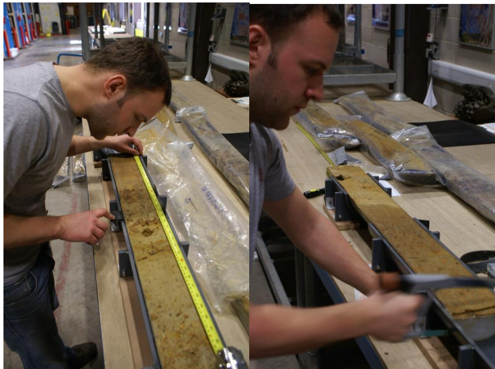
Figure 5.1. a) (left). Removal of core from plastic bag and depth measurement of extracted sample. b) (right). Once sample to be extracted is located a hacksaw is used to separate the sample from the core.
